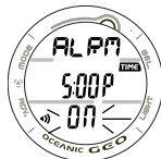
Fig. 21 - DAILY ALARM STATUS
