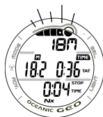
Fig. 84 - DELAYED VIOLATION #2 MAIN
