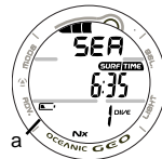
Fig. 3 - LOW BATTERY WARNING
