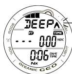
Fig. 85 - DELAYED VIOLATION #3 MAIN
