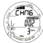
Fig. 4 - LOW BATTERY ALARM
