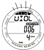
Fig. 87 - VIOLATION GAUGE SURFACE
